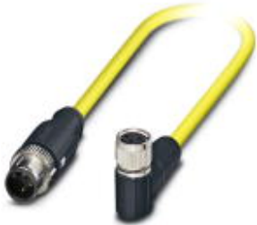
Sensor/Actuator cable, 3-position, PVC, yellow, shielded, Plug straight M12-SPEEDCON, A-coded, on Socket angled M8, Cable length: 1.5 m
